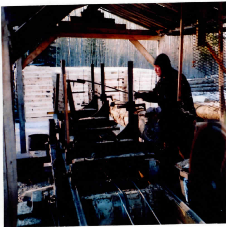
Sawing pipeline skids & bundles of them
